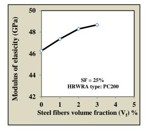
Figure (10) Effect of steel fibers volume fraction on the modulus of elasticity of RPC.
