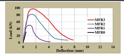
Figure (12) Load-deflection relationship of RPC prisms with Various steel fibers contents.
