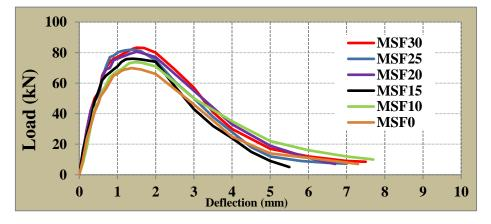
Figure (13) Load-deflection relationship of RPC prisms With various silica fume contents.
