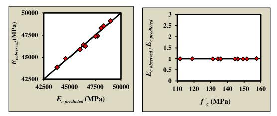
Figure (16) (a) Observed versus predicted values of static modulus of elasticity, (b) The ratio $E_c$  observed  $/E_c$  predicted versus the cylinder compressive strength  $f'_c$ .
