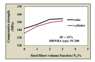
Figure (2) Effect of steel fibers content on cube and cylinder compressive strength of RPC.
