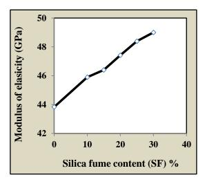
Figure (11) Effect of silica fume content on the modulus of elasticity of RPC.
