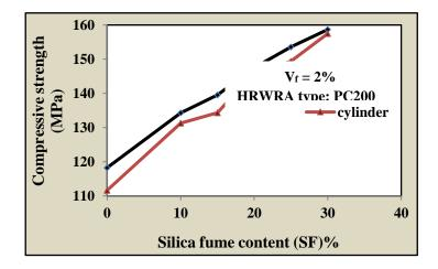
Figure (3) Effect of silica fume content on cube and cylinder Compressive strength of RPC.
