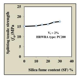
Figure (7) Effect of silica fume content on splitting tensile strength of RPC.
