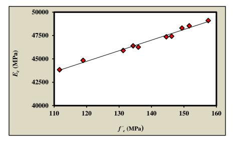
Figure (15) Relationship between compressive strength and static modulus of elasticity for RPC.
