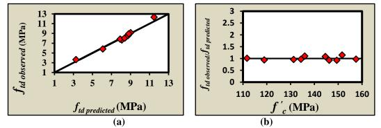
Figure (14) (a) Observed versus predicted values of direct tensile strength, (b) The ratio  $f_{td \ observed} / f_{td \ predicted}$  versus the cylinder compressive strength  $f'_c$ .
