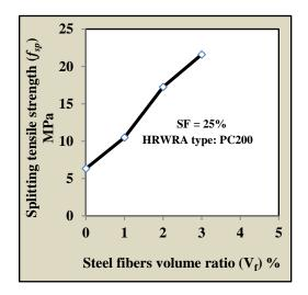
Figure (6) Effect of steel fibers volume fraction on splitting tensile strength of RPC.
