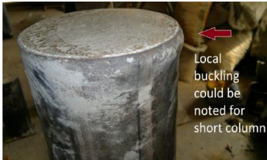
Figure. 7 Failure of the short column.
