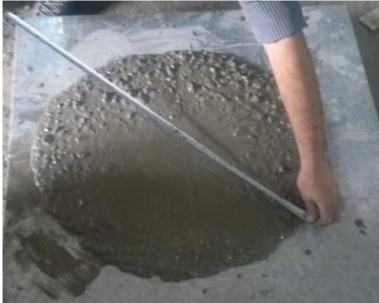
Figure. 1 Slump flow test measurement
