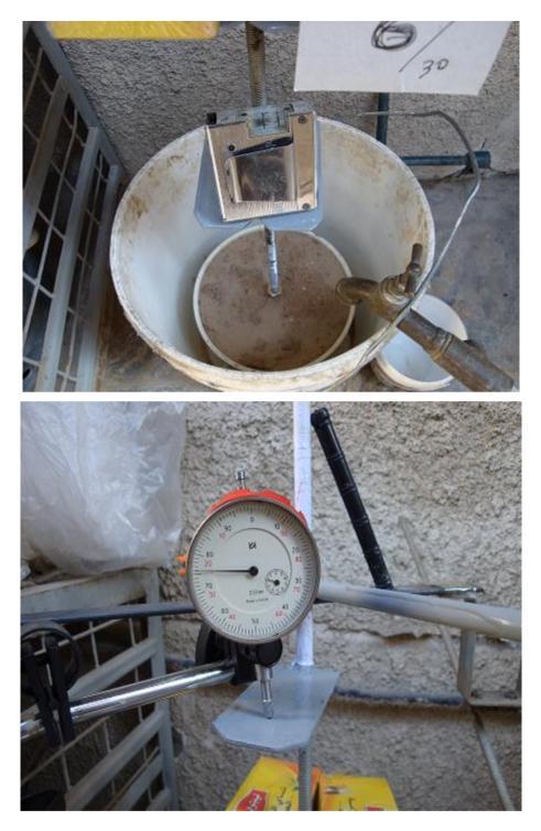
Figure (2-b): Photos showing footing assembly
