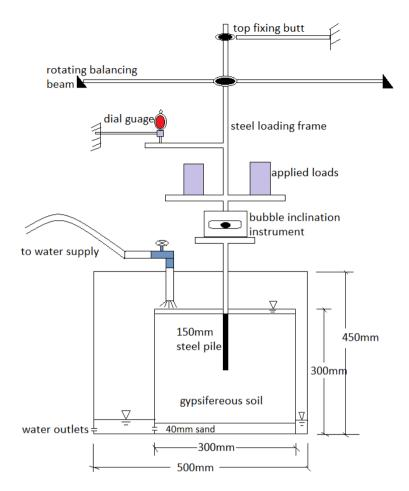
Figure (1): Representative drawing showing testing assembly and loading frame.
