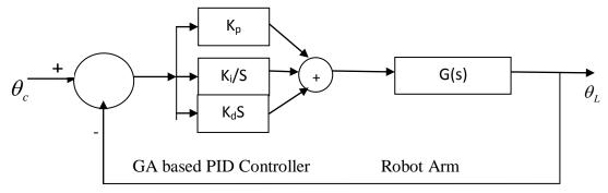
Fig.7. Block Diagram Of The Entire System
