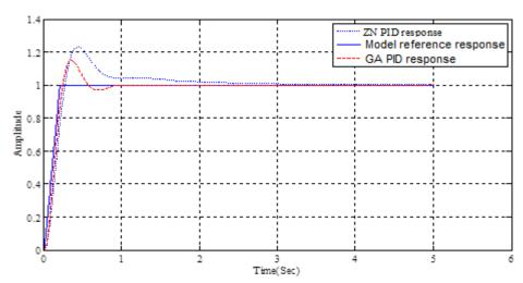
Fig 11. System response under GA-PID controller based on  $G_{m1}$  as a model reference.
