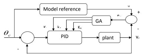
Fig. 10 GA-tuned PID controller based on model- reference approach.
