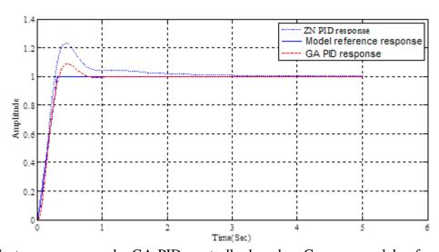
Fig 13. System response under GA-PID controller based on  $G_{m3}$  as a model reference.
