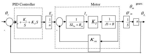
Fig(2). Robot Joint Control System
