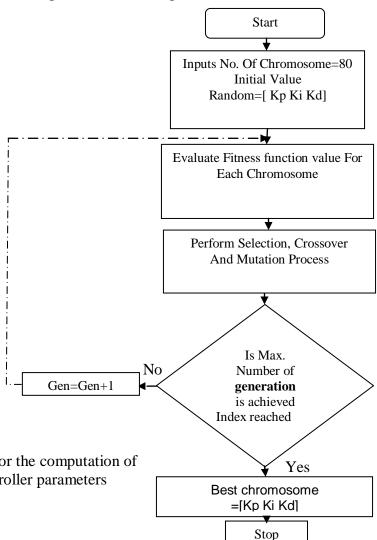
**Fig.5.** Simulation flow chart for the computation of GA-PID controller parameters
