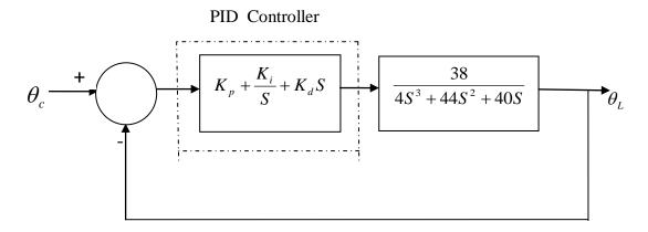
Fig.(3). Joint Control System For A Robot Arm.
