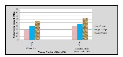
Figure (4) Compressive strength at different ages for normal strength Concrete mixes (not containing HRWRA and silica fume) with and without steel fibers.
