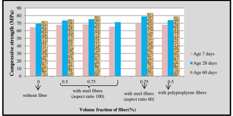
Figure (3) Compressive strength at different ages for HPC mixes with various types, volume fractions and aspect ratios of fibers.
