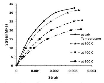
Figure (10) Stress-Strain Relation neither for Normal Concrete NOR at each level of temperature.
