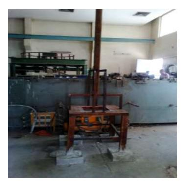
Figure (4) Frame for Impact Resistance Test.
