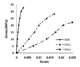
Figure (9) Stress-Strain Relation of Concrete Mixes in Lab Temperature.
