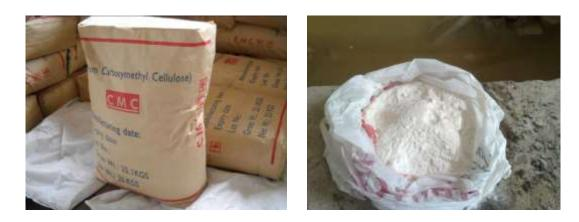
Figure (1) Sodium carboxy-methyl cellulose E466 (CMC).
