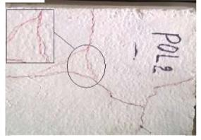
(c) Polymerized Concrete POL2 Figure (16) Failure at Bottom Surface of Concrete Panels.
