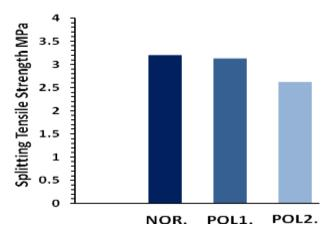
Figure (7) Splitting Tensile Strength of Concrete Mixes in Lab Temperature.
