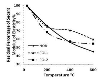
Figure (13) Residual Percentage of Secant Modulus of Elasticity for mixes at each level of temperature.
