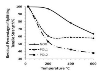
Figure (8) Residual Percentage of Splitting Tensile Strength for mixes at each level of temperature.
