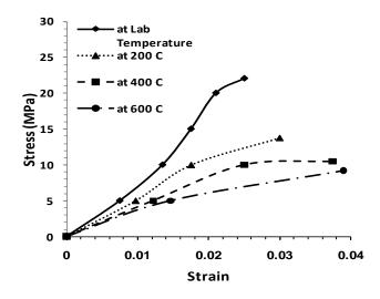
Figure (12) Stress-Strain Relation for Polymerized Concrete POL2 at each level of temperature.
