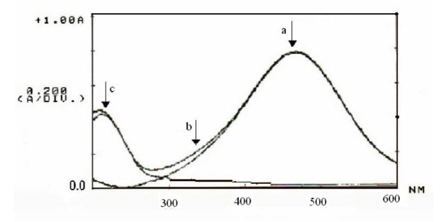
Fig. 2: Absorption spectra of 100 μg of SDZ /25 ml measured against (a) blank,(b) distilled water, and (c) blank measured against distilled water.
