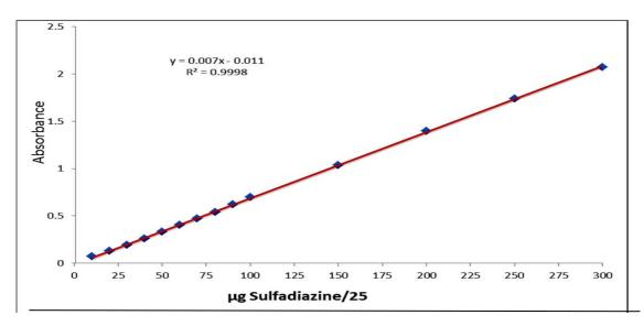
Fig. 1: Calibration curve for sulfadiazine determination , [γ-resorsolic acid] : 0.1%; [NO<sub>2</sub><sup>-</sup>]:1% and [NaOH]: 1M
