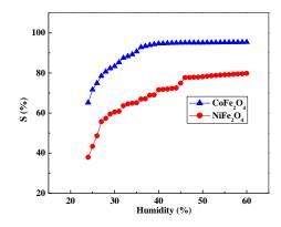
Fig. 6: Variation of sensing response of Co ferrite and Ni ferrite pellet to humidity.
