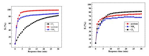
Fig. 4: Sensing response of (a) Co ferrite and (b) Ni ferrite pellet to different gases [acetone, NH<sub>4</sub>, Cl<sub>2</sub>].
