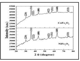
Fig. 1: X-ray diffraction patterns of Ni and Co Ferrites.
