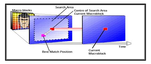
Fig.6: Block Matching Algorithms.
