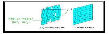
Fig.5: Motion compensation between two frames.
