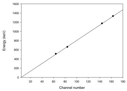
Figure 3: Energy calibration curve of gamma spectrometer.
