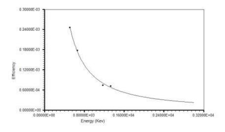
Figure 2: The efficiency calibration curve of gamma spectrometer
