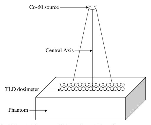
**Fig** (1): Schematic Diagram of the Experimental Procedure.
