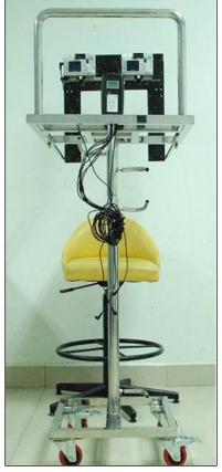
Figure 1. The complete imaging station from frontal view showing the camera base and remote control switch.
