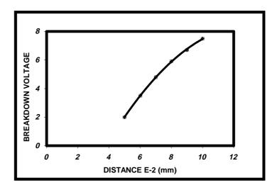
Figure(1): The dependence of breakdown voltage on electrode spacing for Al, Ag and Cu in divergent field conditions
