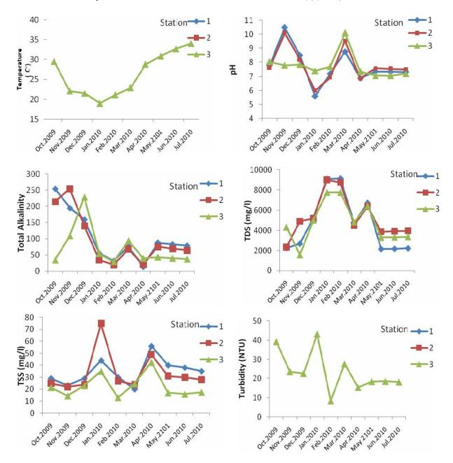
Fig.2: Monthly changes of some wastewater properties (Water temperature, pH, Alkalinity, TSS, TDS and turbidity) within Basra oil refinery treatment system
