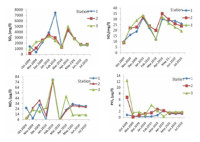
Fig.3: Monthly changes of some wastewater properties (SO<sub>4</sub>, SO<sub>3</sub>, NO<sub>3</sub>, and PO<sub>4</sub>) within Basra oil refinery treatment system
