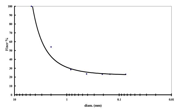
Fig. 1: Gradation of Sand Medium Used in the Studied WTP.
