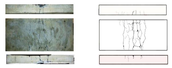
Fig 14: Cracks Pattern of Control Slab (A)
