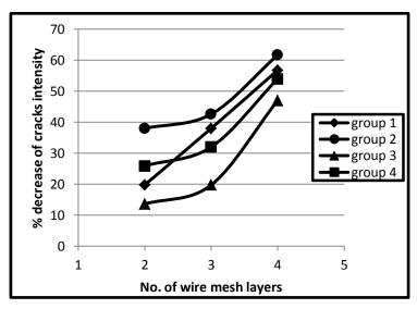
Fig. 15: Effect ofnumber of wire mesh layers on cracks intensity
