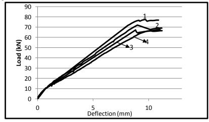
Fig. 8: Load-deflection curve of strengthened slabs
