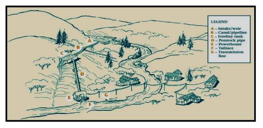
Figure (2): Principal components of a micro-hydropower system [7].
