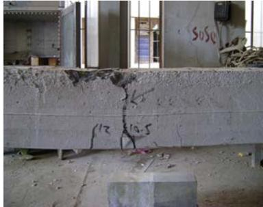
Figure (13) cracks pattern of beam (B1).
