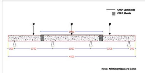
Figure (5) Schematic of specimen B3 with bonded CFRP strip.
