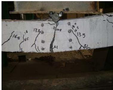
Figure (15) cracks pattern of beam (B2).
