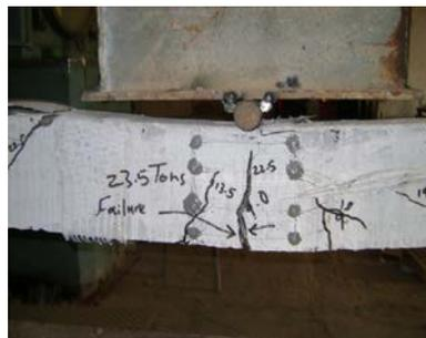
Figure (17) cracks pattern of beam (B3).
