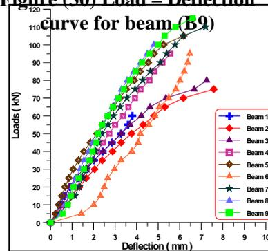
Figure (31) Load Versus Deflection at center of left span for the beams.
