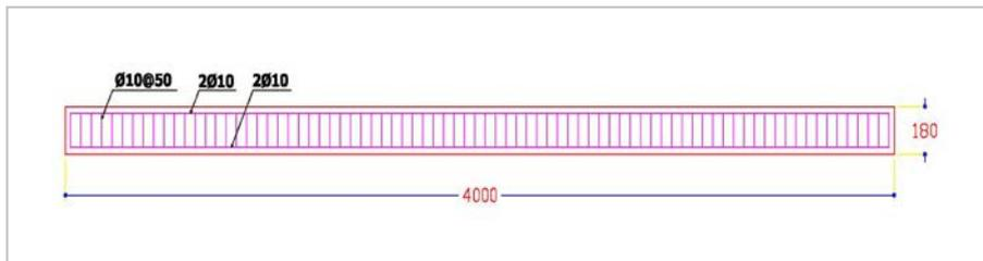
Figure (2) Geometry and reinforcement of the tested RC specimens.
