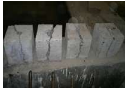
Figure (10) Splitting Failure.
