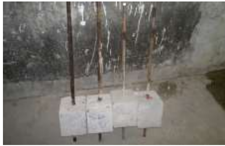
Figure (9) Pull out Failure.
