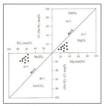
Fig.(4), Groundwater type on Sulin's graph
