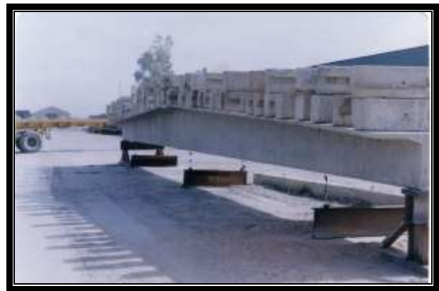
Fig. (6). Beam B1 – Arrangement of the uniformly distributed superimposed dead load
