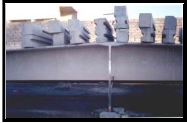
Fig. (14). Beam B2 - Setting the deflection measuring tools.
