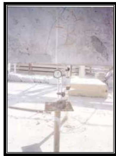
Fig. (20). Beam B3 - Setting up the dial gages
