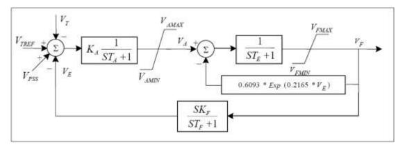
Fig. 3. Block diagram of the excitation system
