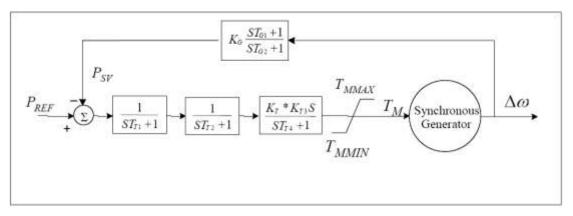
Fig. 2. Block diagram of the turbine and the governor
