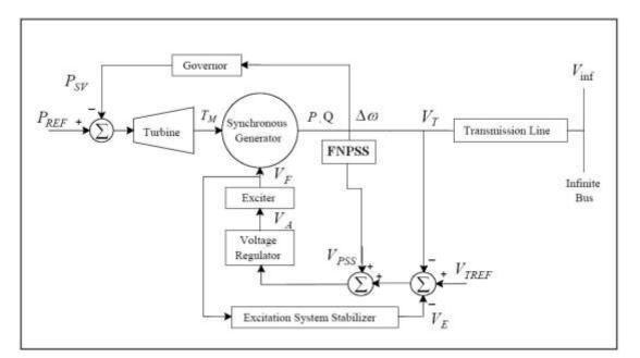
Fig. 1. System model configuration
