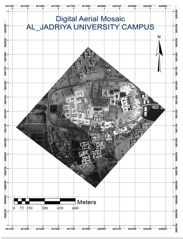
Figure 3. Matching the mosaic of eight digital Arial photos of Baghdad University site by using ERDAS LPS software.
