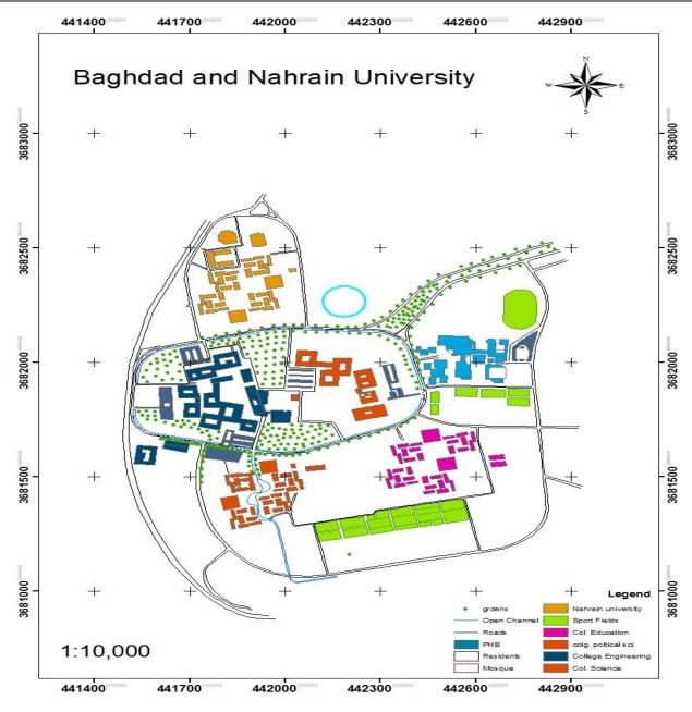
Figure 10. The digital cadastral map of Baghdad University site by using ArcGIS environment, scale 1:10000.
