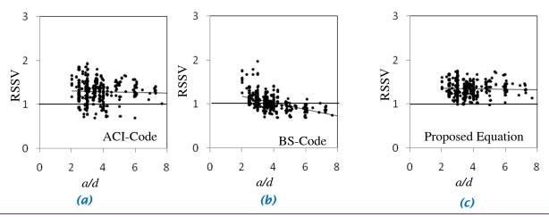
Fig.(4) Shear Span to Depth Ratio Versus the Relative Shear Strength Predictions.
