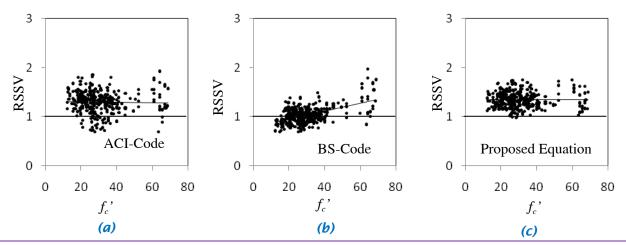
Fig.(2) Concrete Compressive Strength Versus the Relative Shear Strength Predictions.
