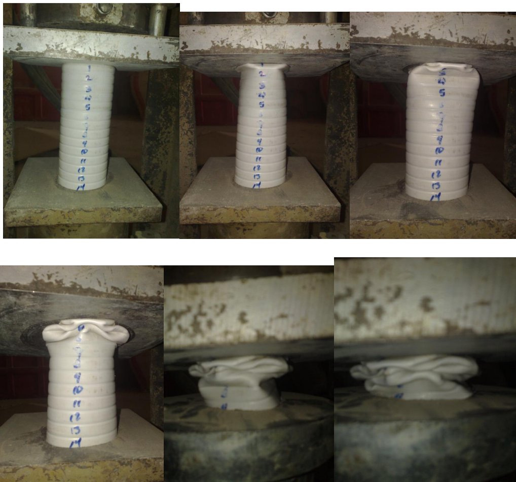
Fig(10): The stages deformation at failure ( complete deflection) for tube with grooved.
