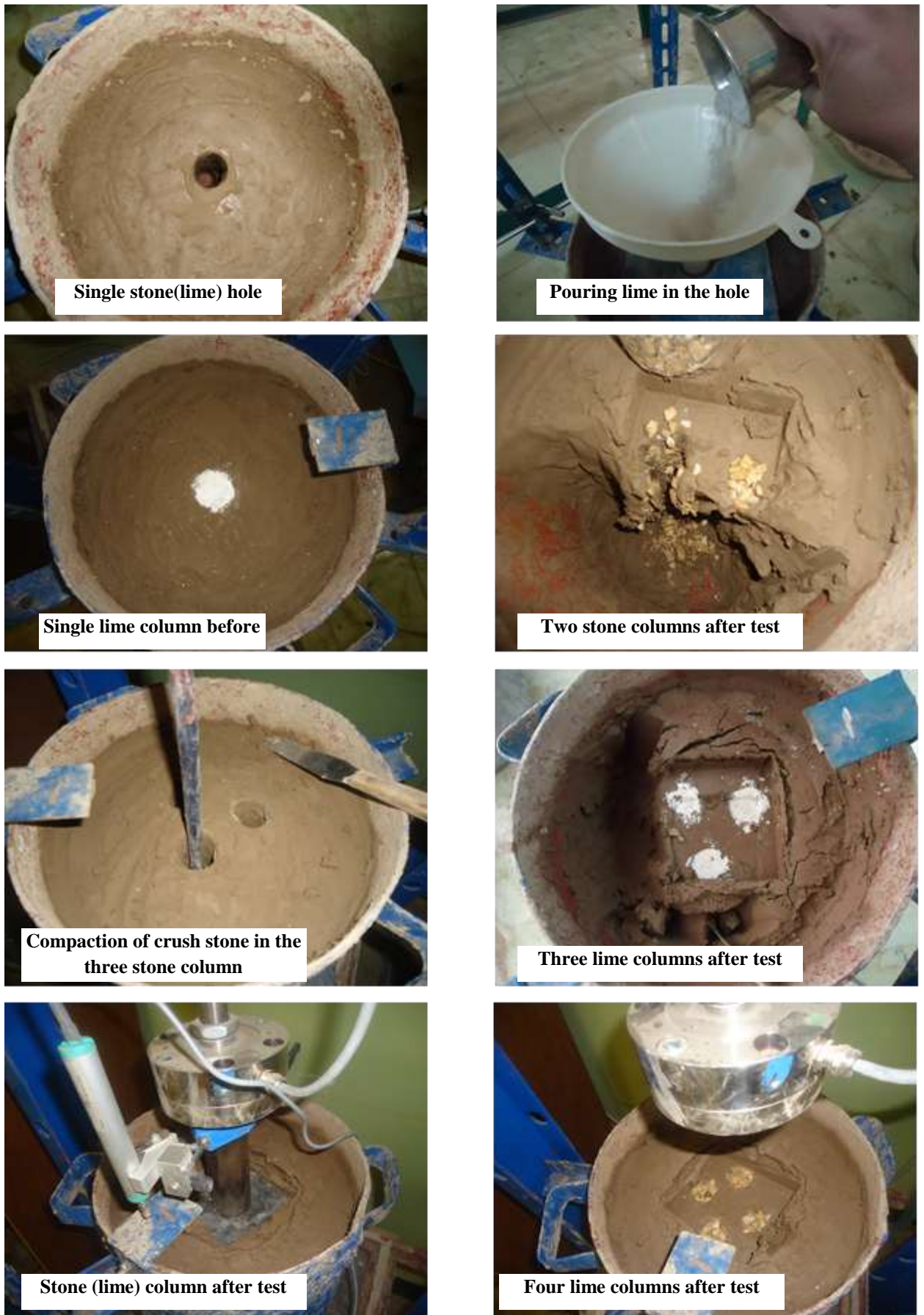
Figure (3) : Stone (Lime) columns before and after tests
