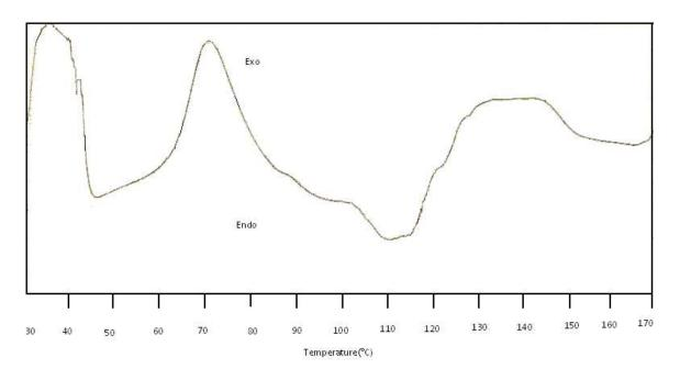
Figure 4: DSC thermogram for esterthioureachloral epoxy:hardner(1:1).
