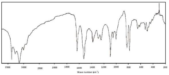
Figure 1: IR spectrum for thioureadichloral.
