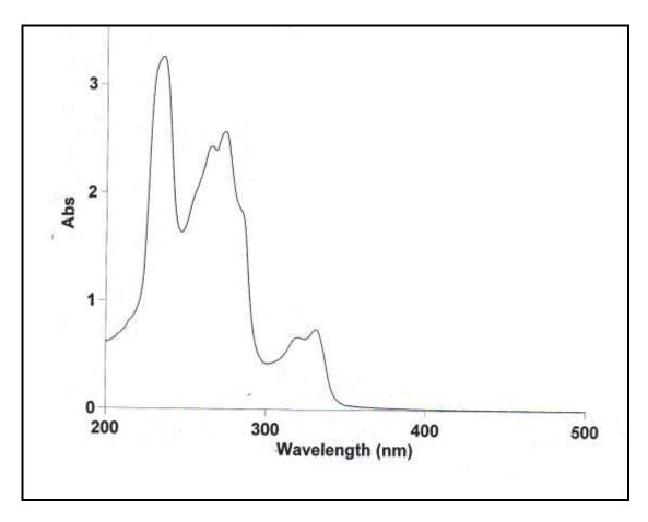
Figure (3): The UV-Vis. spectrum of 1-azo naphthol (2)
