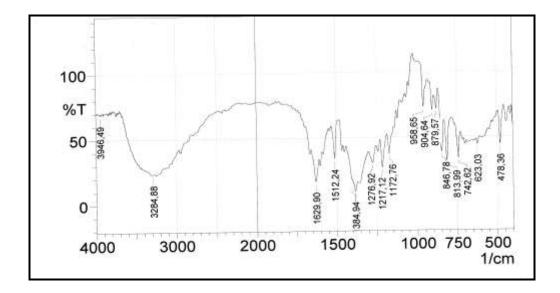
Figure (2): The FTIR spectrum of 1-azo naphthol (2)
