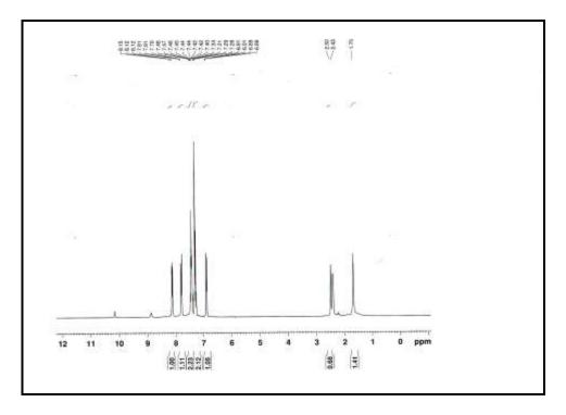
Figure (4): The <sup>1</sup>HNMR spectrum of 1-azo naphthol (2)
