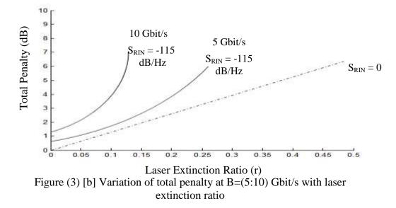
Figs (3-a,b) performance of PIN receiver in the presence of intensity noise
