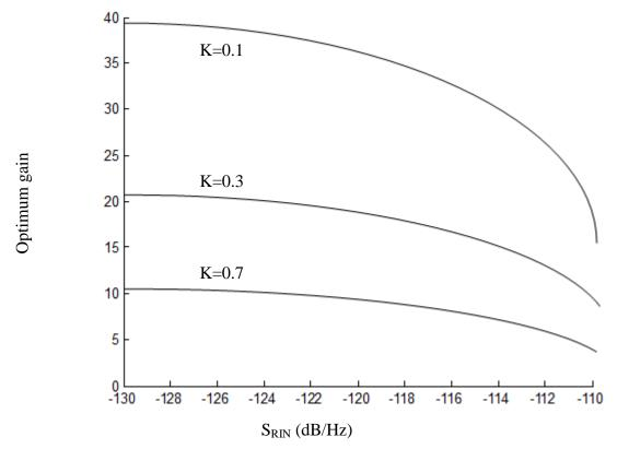
Figure (4) The variation of S<sub>RIN</sub> vs optimum gain
