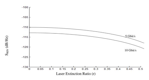
Figure (2) variation of ( $S_{RIN}$ ) at BER=10<sup>-9</sup> with laser extinction ratio
