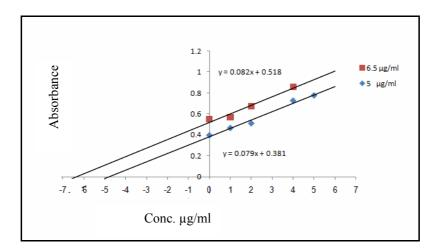
Fig. 6: Graph of standard addition plot for the determination of OMZ in oxymet.
