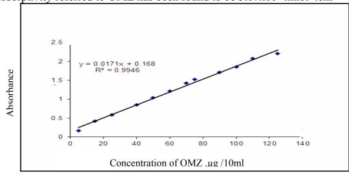
Fig.1: Calibration graph for OMZ determination using the proposed method.
