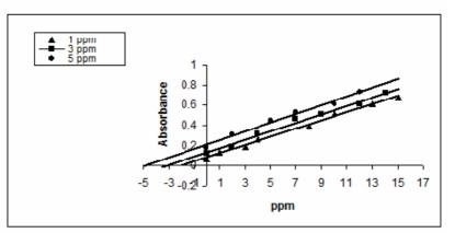
Fig.8 Standard addition plots for the recovery of 1,3,5 µg/ml of sulfacetamide in drop
