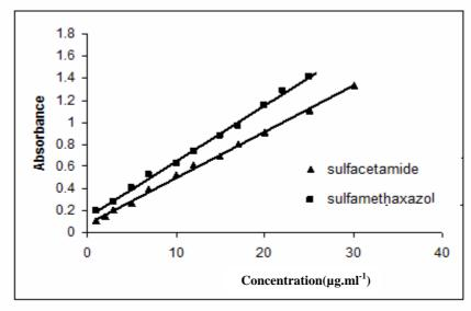
Figure 7. Calibration graphs for (a) sulfacetamide and (b) sulfamethaxazole
