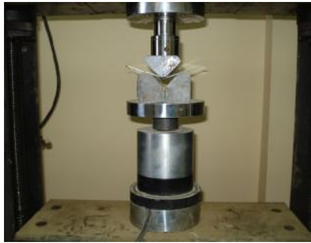
Figure (2) The experimental setup for the V-die bending.
