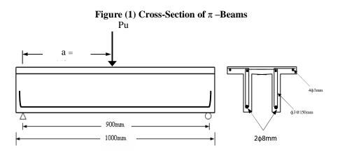
Figure (2) Dimensions and Details of Tested  $\pi$  –Beams
