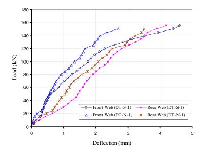
Figure (6) Load-Deflection Curves for Tested Beams (DT-N-1) & (DT-S-1)
