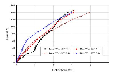
Figure (8) Load-Deflection Curves for Tested Beams(DT-N-4) & (DT-S-4)
