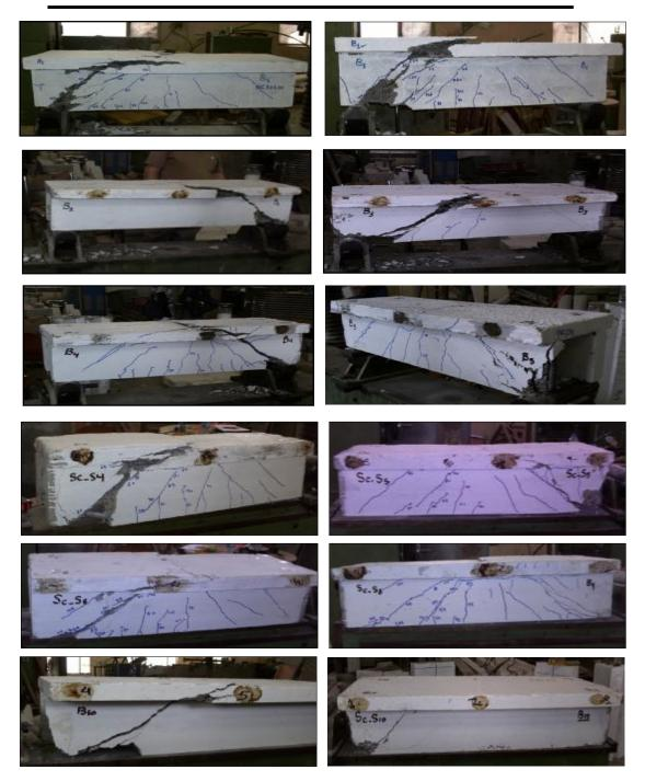
Figure (5) Crack Patterns for double Tee Beams.
