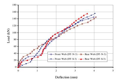
Figure (7) Load-Deflection Curves for Tested Beams(DT-N-3) & (DT-S-3)
