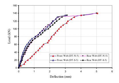
Figure (9) Load-Deflection Curves for Tested Beams (DT-N-5) & (DT-S-5)
