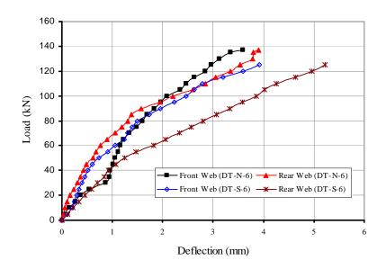
Figure (10) Load-Deflection Curves for Tested Beams(DT-N-6) & (DT-S-6)
