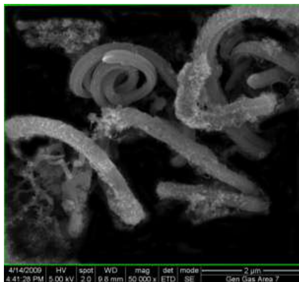
Figure 2: SEM images of the CNFs obtained by \gamma -Fe 2 O 3 catalyst at 400 °C, and (GHSV) 1600 h -1
