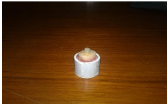
Figure (1) The tooth mounted in polyvinyl plastic ring and the tooth builds up with composite core.
