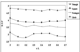
Figure (5): Effect of location of cutout on the S.C.F at  $\theta = 0^{\circ}$ .
