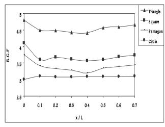
Figure (7): Effect of location of cutout on the S.C.F at  $\theta = 90^{\circ}$ .
