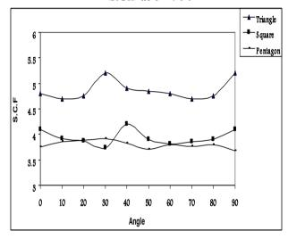
Figure (8): Effect of angle rotation of cutout on the S.C.F.
