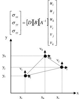
Figure A: Three-nodded triangular plane element [25].
