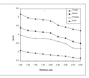
Fig.(10): Effect of thickness on the S.C.F.
