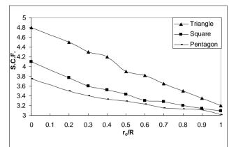
Fig.(9): Effect of sharpness of corner cutout on the S.C.F.
