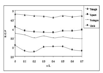
Figure (6): Effect of location of cutout on the S.C.F at  $\theta = 45^{\circ}$ .
