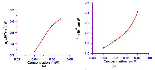
Figure 7 Concentration dependence of (a):  $n_2$ , (b):  $\beta$  of janus green dye in tetrahydrofuran
