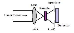
Figure 3 Schematic diagram of experimental arrangement for the Z-scan measurement.
