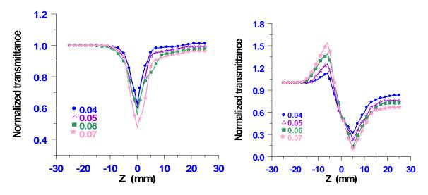
Figure 4 Open-aperture Z-scan data for the THF solution of the azo dye at different concentrations.
