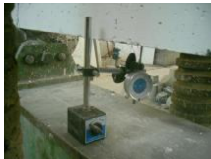
Figure (3) the dial gauge used to record data during testing.
