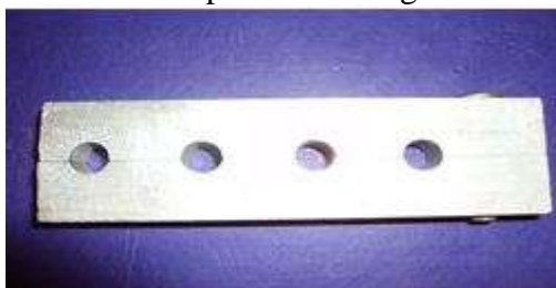
Figure (3):metal pattern for compressive strength.
