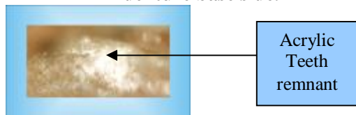
Figure 10: Cohesive failure mode showing acrylic tooth remnants on denture base side.
