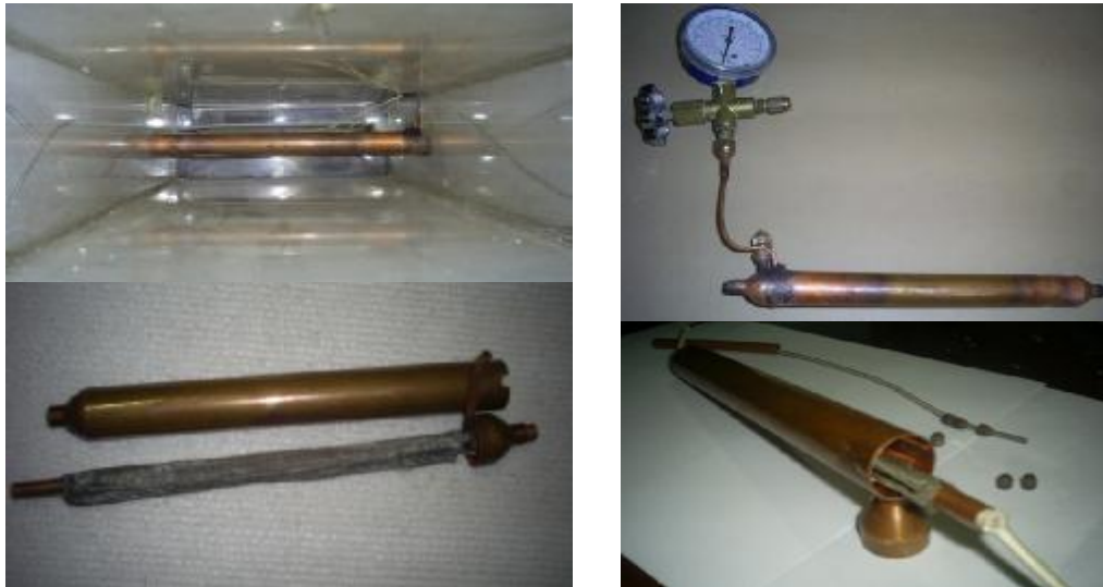
Figure (4) heat valve (HV) construction
