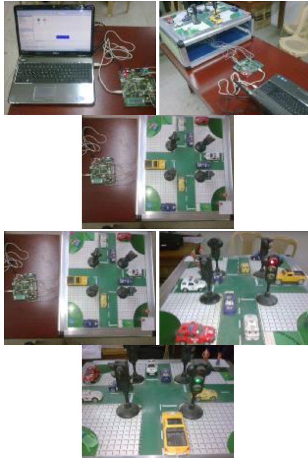
Figure (8) Implementation of the proposed traffic system using the Spartan-3A XC3S700A FPGA kit.
