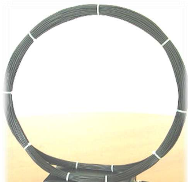
Figure 2. The prototype loop has 40 turns and a diameter of 38 cm
