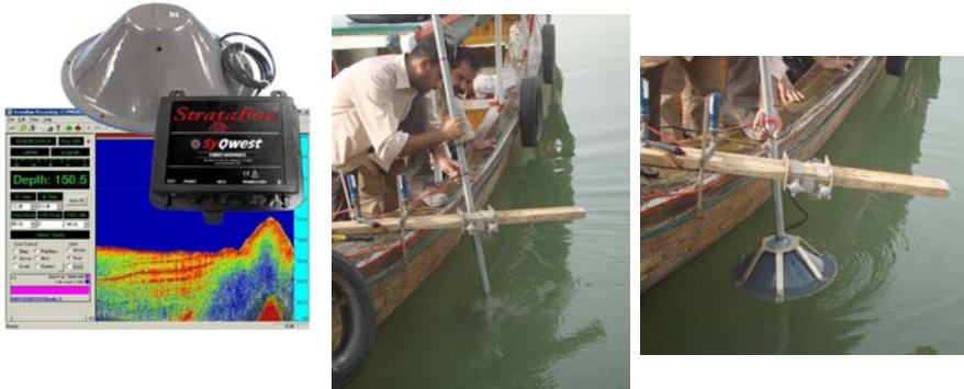
Figure 2. Photos of StrataBox equipment and installation during the field work, the condenser was kept at 0.3 m under the surface of water.
