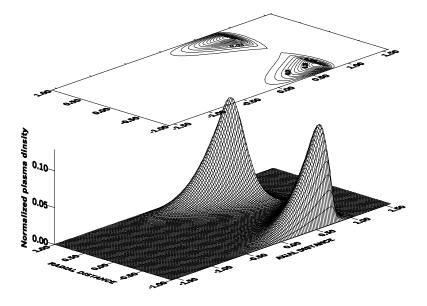
Fig. (6) Two-dimensional distribution of the plasma number density for A cylindrical discharge tube at gas flow velocity (Uo=5.00 m/s.)
