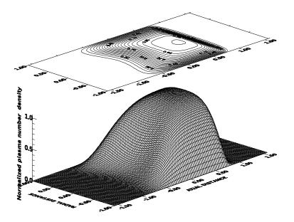
Fig. (3) Two-dimensional distribution of the plasma number density for A cylindrical discharge tube at gas flow velocity (Uo=1.00 m/s.)
