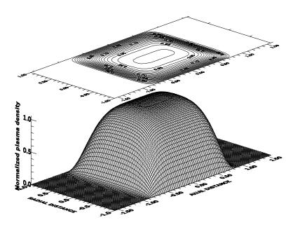
Fig. (2) Two-dimensional distribution of the plasma number density for a cylindrical discharge tube at zero velocity of gas.
