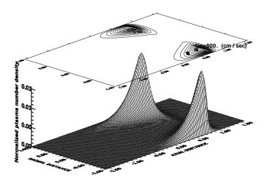
Fig. (7) Two-dimensional distribution of the plasma number density for A cylindrical Discharge tube at gas flow velocity (Uo=8.00 m/s.)
