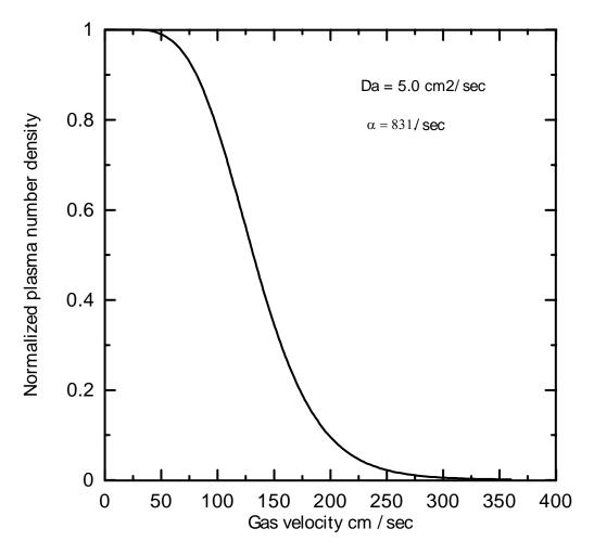
Fig. (9) Normalized plasma number density as a function of gas flow velocity at center cylindrical discharge tube (Z=0, R =0.) for a constants ionisation coefficient and diffusion coefficient
