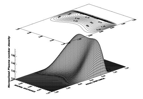
Fig. (4) Two-dimensional distribution of the plasma number density for A cylindrical Discharge tube at gas flow velocity (Uo=2.00 m/s.)
