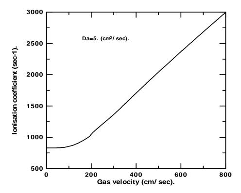
Fig. (8) Ionisation coefficient as a function of gas flow velocity for a cylindrical discharge tube for a constants Normalized plasma number density and diffusion coefficient .
