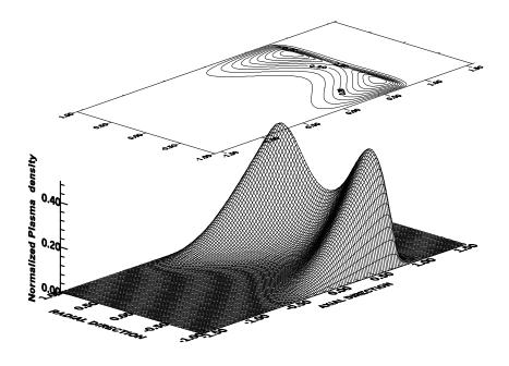
Fig. (5) Two-dimensional distribution of the plasma number density for A cylindrical Discharge tube at gas flow velocity (Uo=3.00 m/s.)
