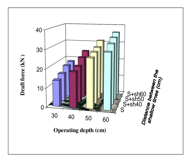
Figure (3): The draft force versus the operating depth for different lateral distance between the shallow tines.
