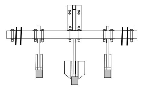
(B) Front view Figure (1) The subsoiler with shallow tines. 2.2 The draft force measurement
