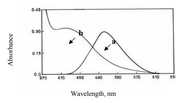
Fig.1 Absorption spectra of (a) 75µg trifluoperazine hydrochloride with sulfanilic acid against reagent blank, and (b) reagent blank versus distilled water.
