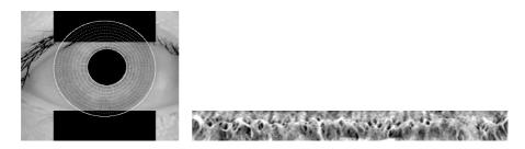
Fig. (6): The Cartesian and polar coordinates of an iris
