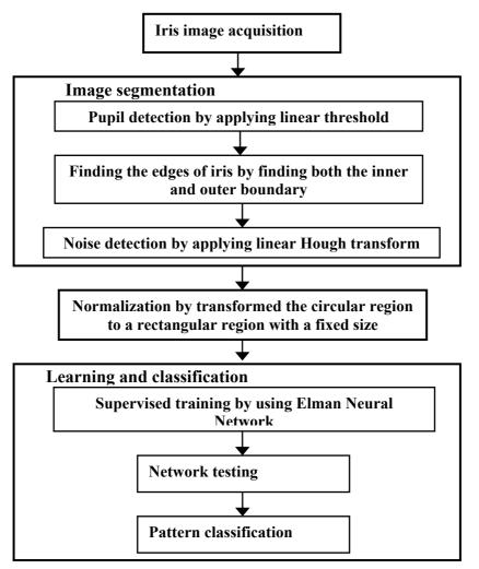
Fig. (2): The structure of the iris recognition system
