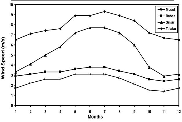
Fig (6) : Monthly Mean Wind Speed (m/s) at 50 m for all Stations
