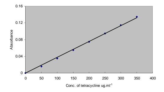
Fig. 3 : Calibration curve for determination of tetracycline by spectrophotometric method
